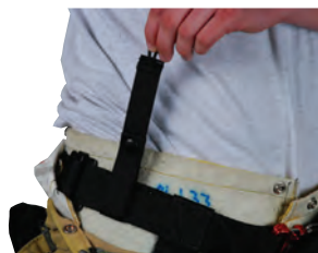
Harness keeper tab snaps around waist belt of harness.
