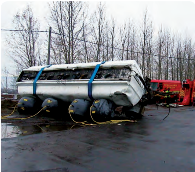
Efficient lifting of overturned vehicles.
