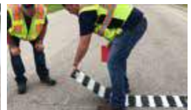
Chalk outline indicates insignificant movement observed after repeated roll over and braking
